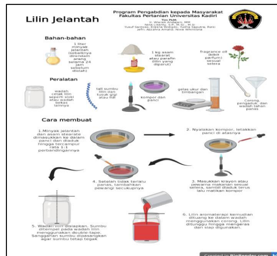
Figure 1. Brochure or Pamphlet of Step-by-Step Making an Aromatic Candle Using Used Cooking Oil
