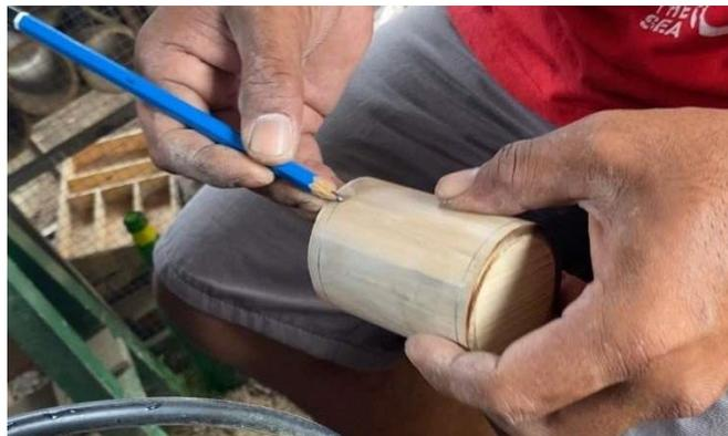
Gambar 7. Proses Sketsa Bambu
