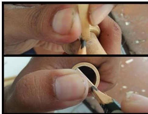
Figure 3. Determining the flute diameter
