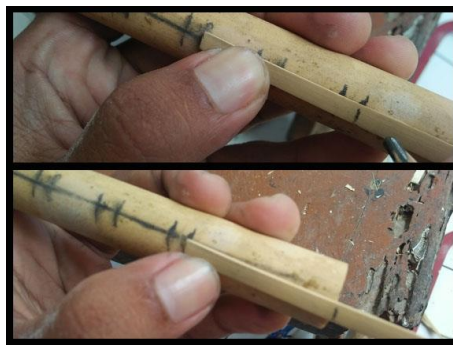
Figure 4. Measuring distance of finger hole and bottom of flute
