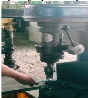
Gambar 9. Proses *chamfering*
