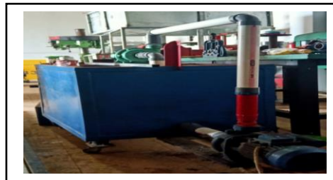
Figure 3. A laboratory Scale Pump as Turbine (PAT)
