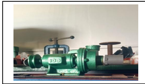
Figure 2. Pump as Turbine That Has Been Installed
