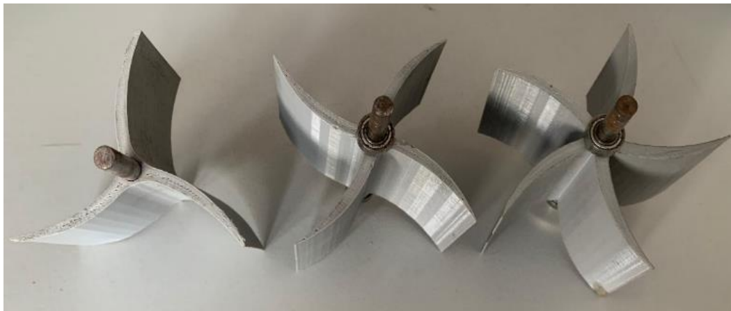
Figure 3. Cooling Fan with 3 Blade, 4 Blade, and 5 Blade Variations
