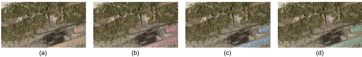
Figure 7. Results of hole detection in mulch in area 3 before overlay using (a) Template Matching and after overlay using (b) Random Forest, (c) Support Vector Machine, and (d) XGBoost
