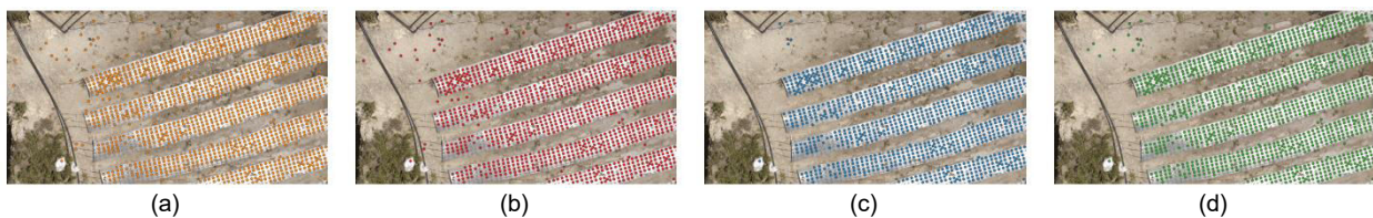
Figure 10. Results of hole detection in mulch in area 6 before overlay using (a) Template Matching and after overlay using (b) Random Forest, (c) Support Vector Machine, and (d) XGBoost
