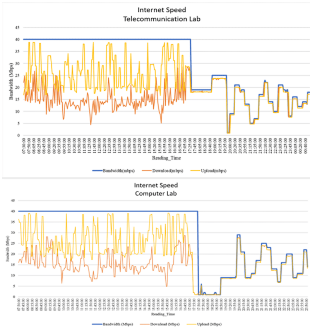
Figure 4. Effect of Elastic WLAN on Upload rate and Download rate on both rooms
