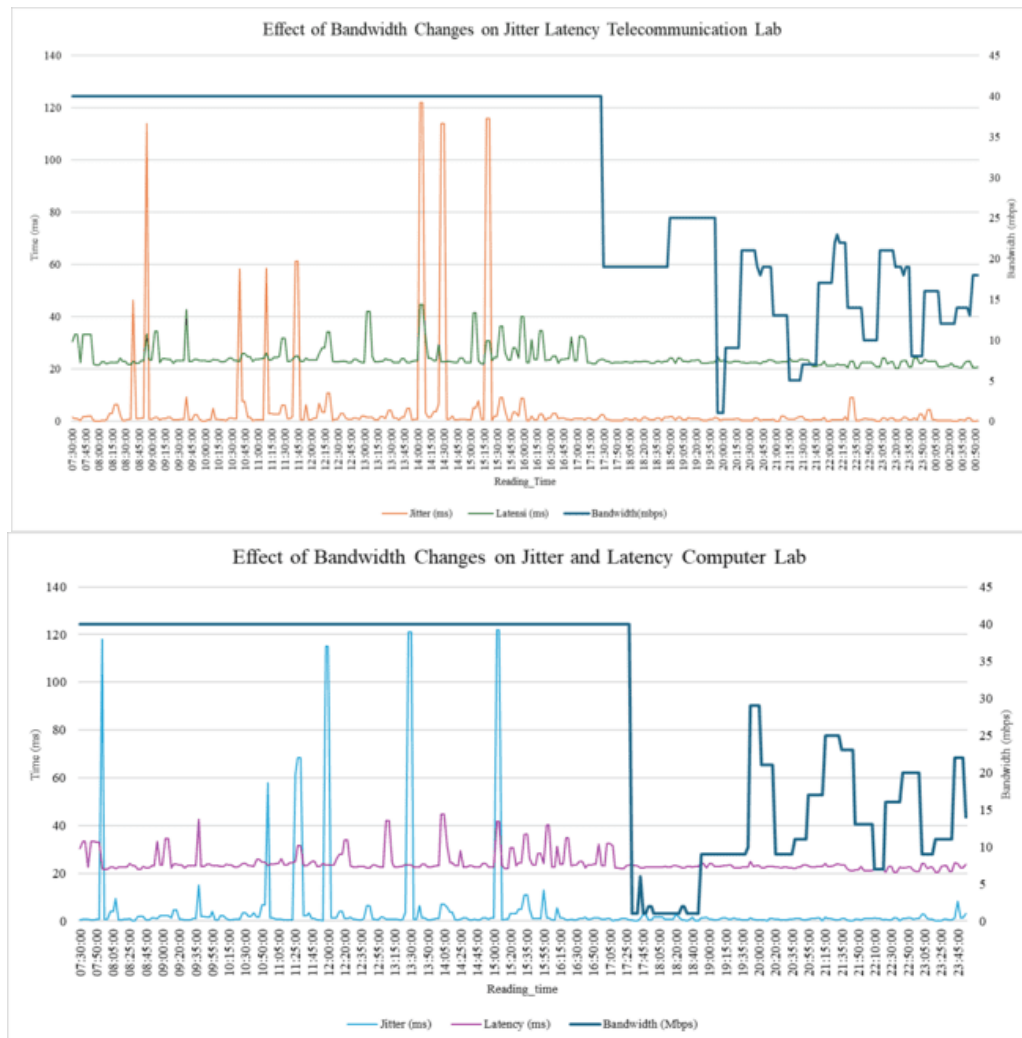
Figure 5. The Effect of Elastic WLAN on Jitter and Latency in Both Rooms
